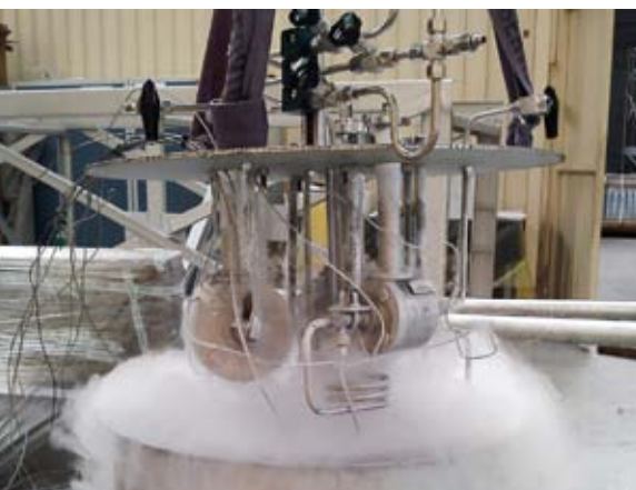
Leakage test at very low temperature
